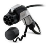
AC charging cable, AC charging cable with Vehicle Connector, open cable end, with locking option for U-lock, with protective cap, C-Line black / gray, GB/T, GB/T 20234.2-2015, GB/T 18487.1-2015, 32 A / 440 V (AC), design line C-Line, cable: 5 m, black, straight, mating face: black, handle area: gray
