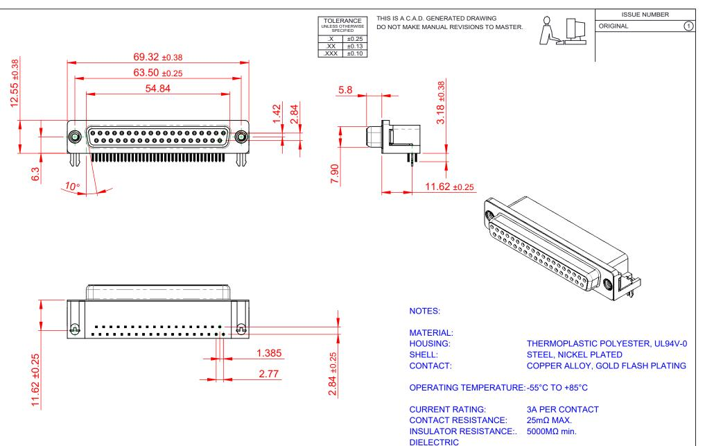
WITHSTANDING VOLTAGE: 1000V AC rms
