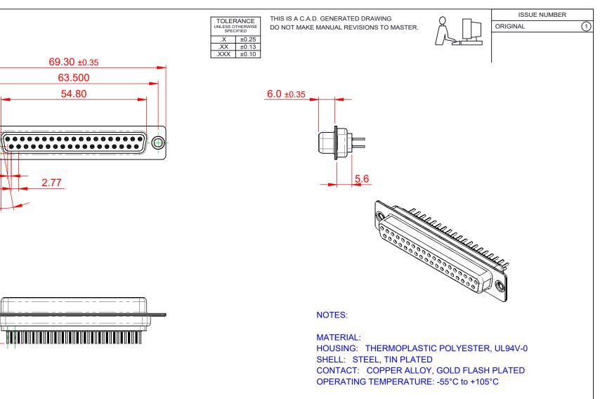
CURRENT RATING: 3A PER CONTACT CONTACT RESISTANCE: 25mΩ MAX. INSULATOR RESISTANCE: 5000MΩ min. DIELECTRIC WITHSTANDING VOLTAGE: 1000V AC rms
