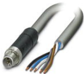
Power cable, 5-position, PVC, gray RAL 7001, Plug straight M12, L-coded, on free cable end, cable length: 5 m, for direct current up to 16 A/63 V
