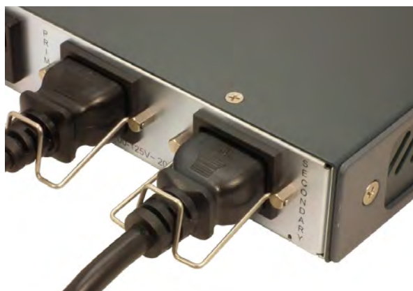
Figure 3-7 AC Power Input
