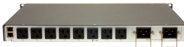
Figure 3-8 100-120 VAC SLB - Branch Office Manager Power Outlets
