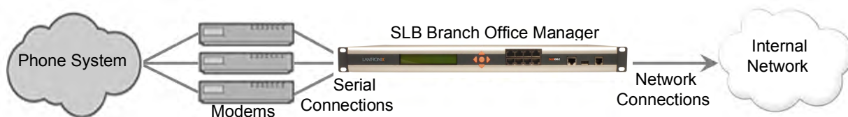
Figure 10-2 Remote Access Server
