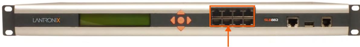
Figure 2-6 Device Port Connections
