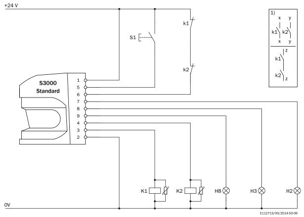
S3000 Standard in conjunction with relays/contactors
