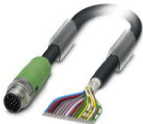
Sensor/actuator cable, 17-position, PUR/PVC, black RAL 9005, shielded, Plug straight M12 SPEEDCON, A-coded, on free cable end, cable length: 10 m
