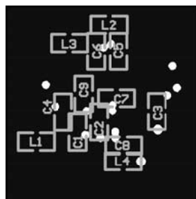
Figure 25. Bottom Layer Silkscreen
