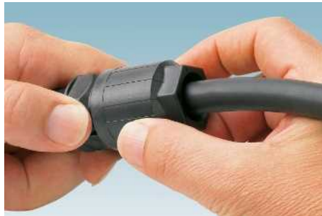
5. You will feel the wires engage when they have reached the optimum screw-on width. The QUICKON nut is now screwed on so tight that it cannot be unscrewed again by hand.
