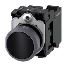
Pushbutton, 22 mm, round, plastic with metal front ring, black, pushbutton, flat, momentary contact type, with holder, 1 NO, spring-type terminal, with laser labeling, upper case
