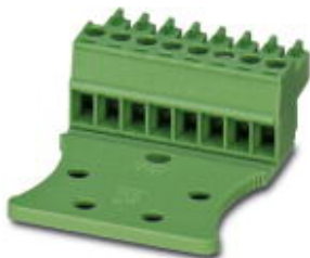
PCB connector, nominal current: 8 A, number of positions: 8, pitch: 3.5 mm, connection method: Screw connection with tension sleeve, color: green, contact surface: Tin
