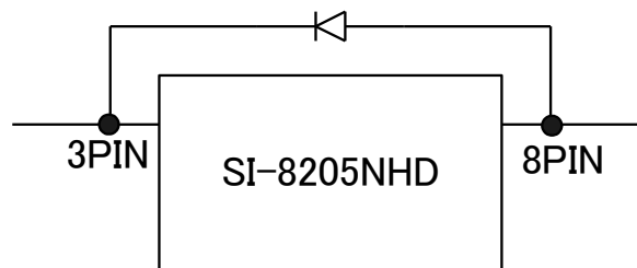
Fig. 23 Diode for Reverse Bias Protection
