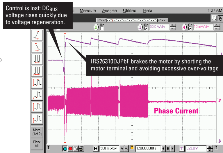
DC Bus over-voltage protection scheme in IRS2631DJ
