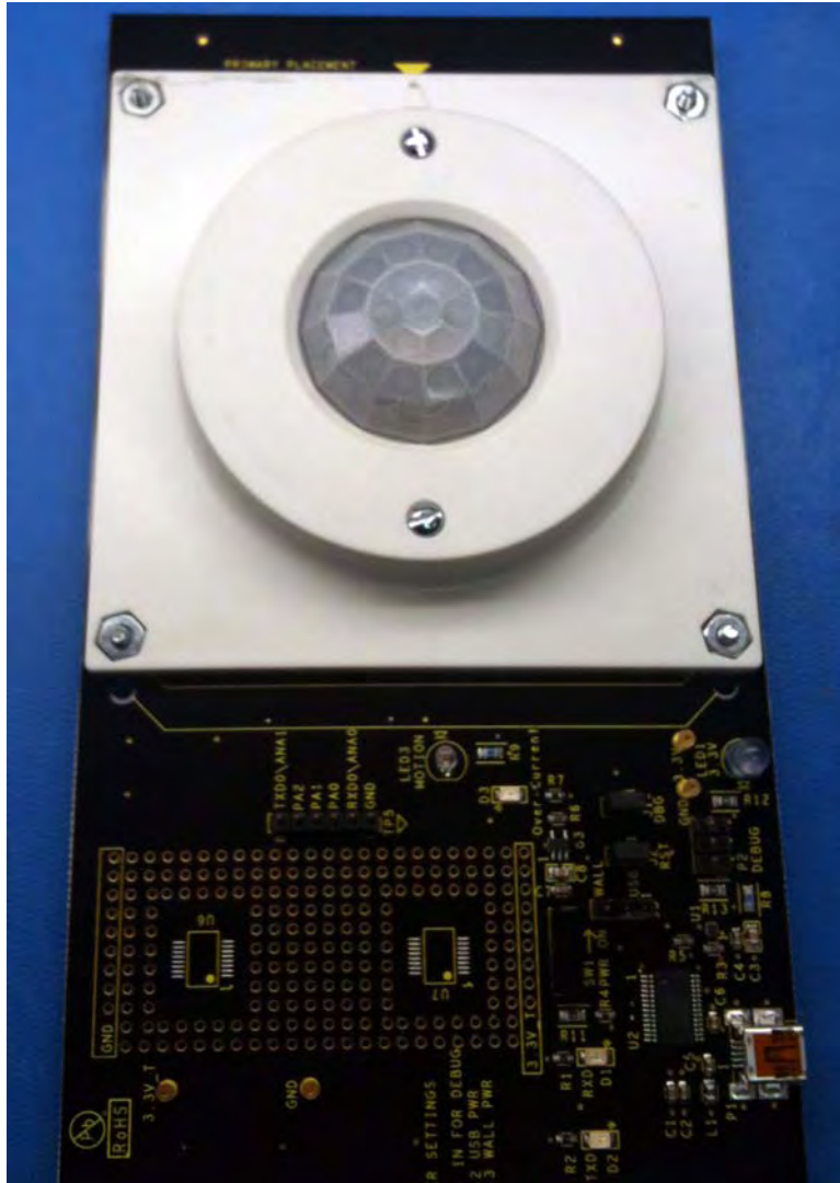
Figure 7. Assembled Circular 0.77" Lens Holder and Circular Lens Installed on the ZMOTION Development Board
