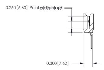
745 Series Ultra-Mate Card Edge Connector - Press Fit REAVANT Part Number: 745-051-540-106 **EDAC INC** THESE DRAWINGS AND SPECIFICATIONS ARE THE PROPERTY OF EDAC INC., AND
