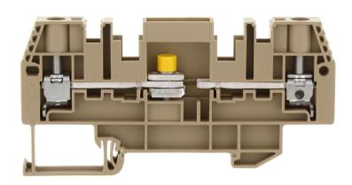
Test disconnect terminal, Screw connection, Mounting type: Mounting rail TS 35/7.5, Rated cross-section: 6 mm², Width: 8.1 mm, Colour: Beige
