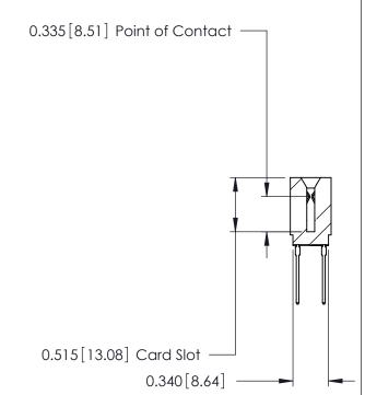
746 Series Ultra-Mate Card Edge Connector - Press Fit Part Number: 746-052-545-201
