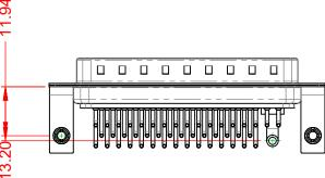
POWER/CO-AX CONTACT RATING: (IF PRESENT) SIGNAL CONTACT CURRENT RATING: 5A PER CONTACT SIGNAL CONTACT RESISTANCE:  $10m\Omega$  MAX. **INSULATOR RESISTANCE:**
