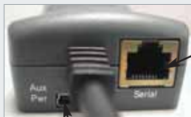
Auxiliary Power Connector (for optional power cable)
