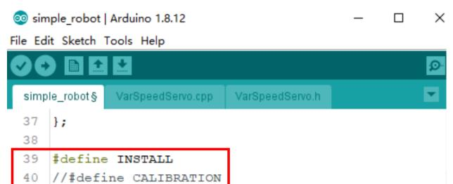
Note: Only one function can be used at the same time. Starting multiple functions might break down the robot.
