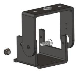
Use the same method to secure the other round hole on the 4th and 5th boards, as shown in the following figure:
