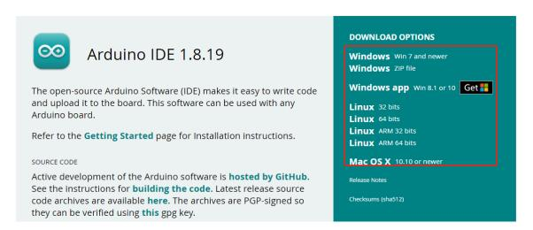
There are two versions of Arduino for Windows: Installer or ZIP file. You're recommended to download the former. Just download the package, and run the executable file to start installation. It will download the driver needed to run Arduino IDE. After downloading, follow the prompts to install. After installing, you will see Arduino icon on your desk and double click to open it.
