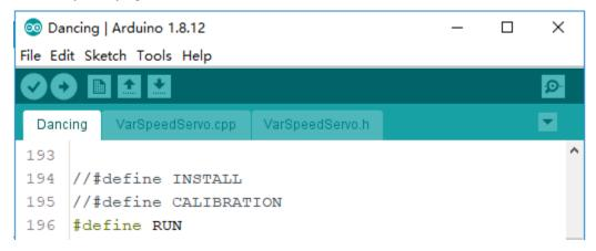
After burning successfully, unplug the USB cable and press the power button on the servo control board. You will see the robot dancing.
