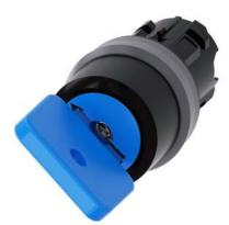
Key-operated switch O.M.R, 22 mm, round, plastic with metal front ring, lock number 73038, blue, with 2 keys, 2 switch positions O-I, latching, actuating angle 90°, 10:30h/13:30h, key removal O+I, with laser labeling, upper case and lower case, always upper case at beginning of line
