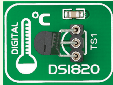
Figure 20-2: DS1820 correctly placed in socket
