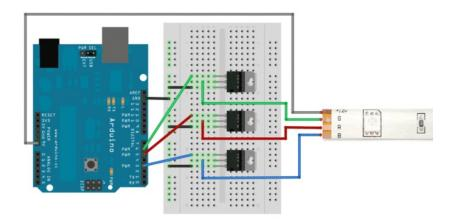
This diagram shows connecting up with power NPN transistors such as TIP120, where Base is pin 1, Collector is pin 2 and Emitter is pin 3. Its very similar except this time we have 100-220 ohm resistors between the PWM output pin and the base.
