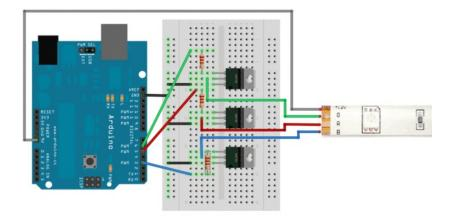
Connect a 9-12V power supply to the Arduino so that **Vin** supplies the high voltage to the LED strip. If you want, you can also just use a separate wire that connects to a power supply that provides about +12V. Make sure to connect the ground of that supply to the ground of the Arduino/MOSFETs!
