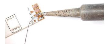
Solder the four wires on. We used stranded wire, which is more flexible and is probably a better choice than solid-core.
