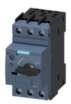
Circuit breaker size S0 for system protection without phase failure protection A-release 10...16 A N-release 208 A screw terminal Standard switching capacity
