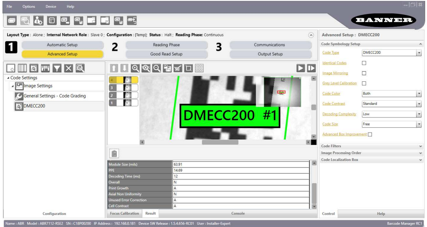
Figure 168. Select a Code Type on the Code Settings Page to View Code Grades from the Result Tab
