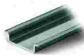
Item no.: 210-113 Steel carrier rail; 35 x 7.5 mm; 1 mm thick; 2 m long; unslotted; according to EN 60715; silver-colored
