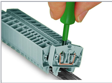
Remove terminal block from the DIN-rail with a levering action.
