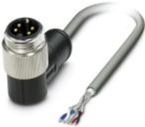
Bus system cable, DeviceNet, 5-position, PUR halogen-free, Gray RAL 7001, Plug angled 7/8"-16UNF, on Free cable end, Cable length: 10 m
