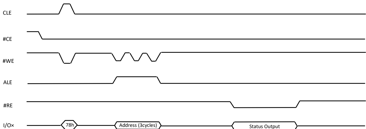
Figure 9-7 Read Status Enhanced (78h) Operation
