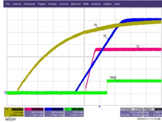
Fig. 8. Start up at 3A Load, Ch 1 :V in , Ch 2 :V o , Ch 3 :V ss , Ch 4 :V PGood
