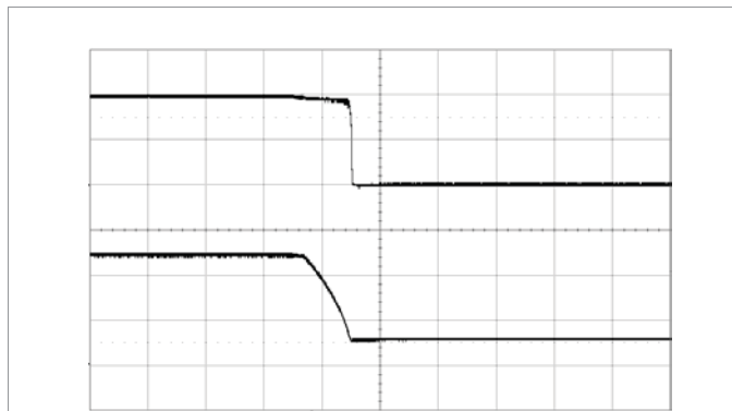
Shut-down enabled by disconnecting V_I at: T_{P1} = +25\text{ }^\circ\text{C} , V_I = 12\text{ V} , V_O = 1.0\text{ V} C_O = 470\text{ }\mu\text{F}/10\text{ m}\Omega , I_O = 20\text{ A} Top trace: output voltage (0.5 V/div.). Bottom trace: input voltage (5 V/div.). Time scale: (2 ms/div.).
