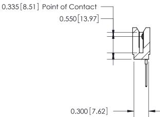
745 Series Ultra-Mate Card Edge Connector - Press Fit Part Number: 745-054-545-106 THESE DRAWINGS AND SPECIFICATIONS
