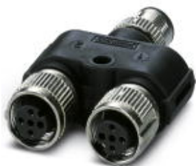
Y distributor, 3-position, unshielded, Plug straight M12 SPEEDCON, A-coded, on Socket straight M12 SPEEDCON, A-coded and Socket straight M12 SPEEDCON, A-coded, with 3 LEDs
