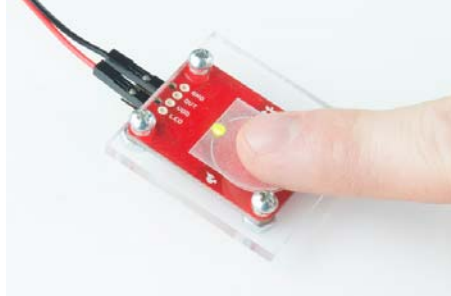
The AT42QT101X will detect touch through 0.125 inch acrylic
