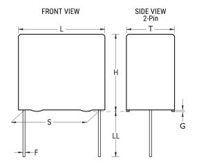
**General Information** Series PFR/F411 Dielectric Film/Foil Polypropylene Style Radial Features Pulse RoHS Yes Wire Leads Lead AEC-Q200 No Component 0.414 g Weight An Operating Temperature Up To +105C Is Allowed Under Certain Conditions. Please Consult Miscellaneous KEMET For Details.
