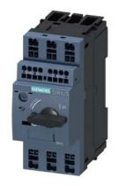
Circuit breaker size S00 for motor protection, CLASS 10 A-release 0.18...0.25 A N-release 3.3 A Spring-type terminal Standard switching capacity with transverse auxiliary switches 1 NO+1 NC
