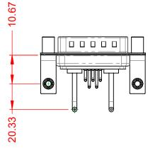
10A (CURRENT) POWER/CO-AX CONTACT RATING: (IF PRESENT) SIGNAL CONTACT CURRENT RATING: 5A PER CONTACT SIGNAL CONTACT RESISTANCE:  $10m\Omega$  MAX.
