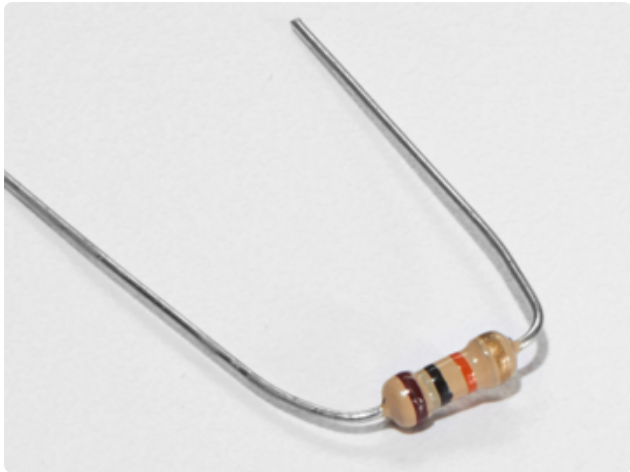
10K Ohm Resistor Colors: Brown > Black > Orange
