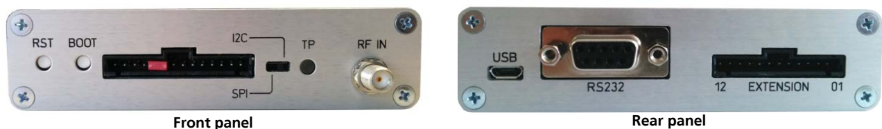
Figure 2: EVK-M8F-0-00 evaluation unit – front and rear panels
