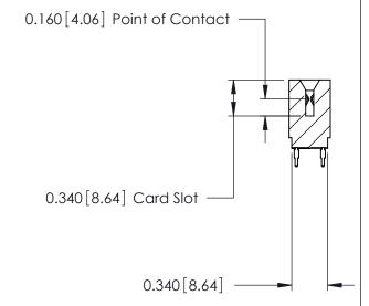
ACAD REFERENCE NO. 746 Series Ultra-Mate Card Edge Connector - Press Fit DRAWN: Part Number: 746-074-525-601 CHECKED: **EDAC INC** SCALE: THESE DRAWINGS AND SPECIFICATIONS ARE THE PROPERTY OF EDAC INC.,AND
