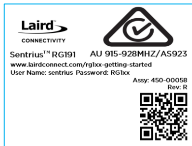
Figure 82: Australia 915 or 923MHz Region Supported Label (Frequency changes depending on setting)
