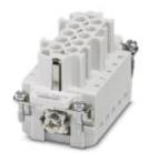
Contact insert, number of positions: 10+PE, size: B10, number of connections per position: 2, Socket, Push-in connection, 500 V, 10 A, 0.25 mm² ... 1.5 mm², application: Power
