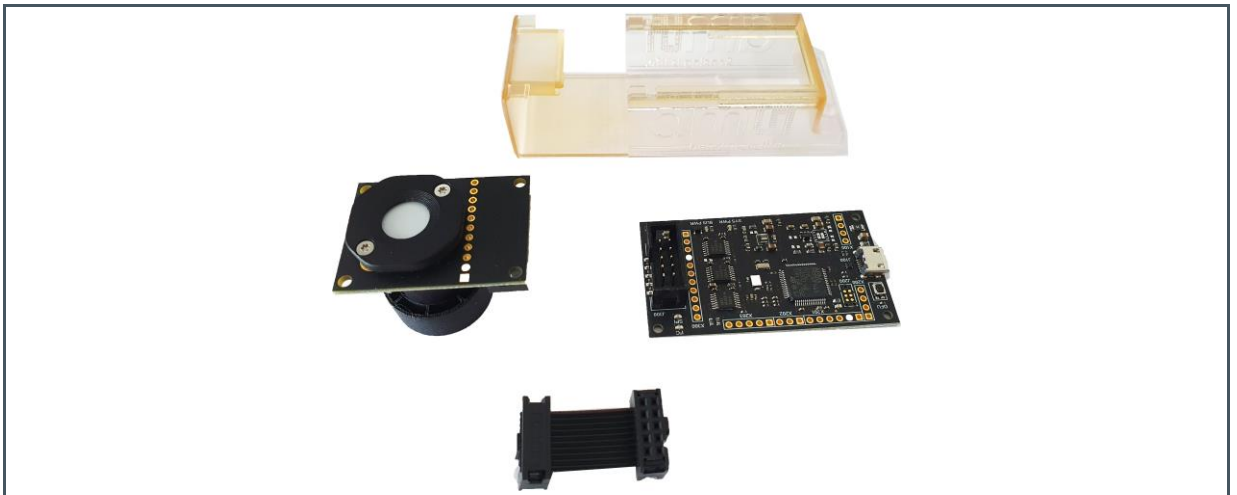
Figure 6: Sensor and Standard Unicom Board Connected via Ribbon Cable, USB-Interface, and an Insertable Plastic Housing
