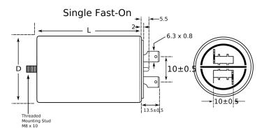
Series C27 Dielectric Film/Foil Polypropylene Style Plastic Case and Cover, Ultra Sonically Welded Description Ultra Sonically Welded Seal, Safety Class PO, Features UL 94 V0 Disk **RoHS** Yes Lead Fast On (1+1) UL, VDE, UL (Construction Only), UL\_94 VO Qualifications Disk AEC-Q200 No Component 142 g Weight
