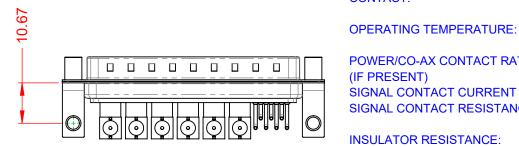
75Ω (IMPEDANCE) POWER/CO-AX CONTACT RATING: (IF PRESENT) SIGNAL CONTACT CURRENT RATING: 5A PER CONTACT SIGNAL CONTACT RESISTANCE:  $10m\Omega$  MAX. **INSULATOR RESISTANCE:** 5000MΩ min.
