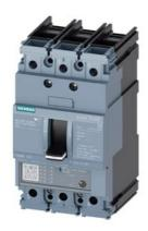
circuit breaker 3VA5 UL frame 125 3-pole, starter protection TM120M, AM, In=40A without overload protection short-circuit protection li=5...12 x In cable connection on both sides
