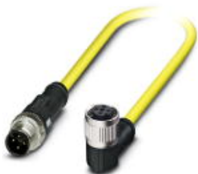
Sensor/actuator cable, 4-position, PVC, yellow, Plug straight M12 SPEEDCON, A-coded, on Socket angled M12 SPEEDCON, A-coded, cable length: 0.5 m
