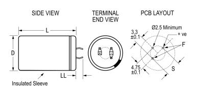
General Information Series ALC80 Dielectric Aluminum Electrolytic Description Snap-In, Aluminum Electrolytic RoHS Lead 3 Pin Short AEC-Q200 No Halogen Free Yes Component Weight 55 g Notes Dimensions D And L Include Sleeving. Shelf Life 156 Weeks
