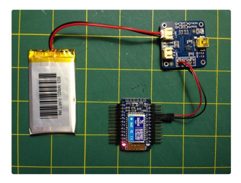
Let's test to make sure we're getting power from the battery through the charge controller to the EZ-Key.
