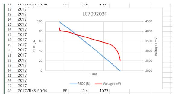
This graph shows association between time and cell voltage and RSOC in constant current discharging.
